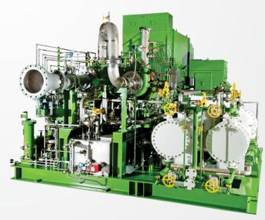
The two-stage MSG-7 compressor pictured above handles propane in a refrigeration loop at a refinery in South Korea.
